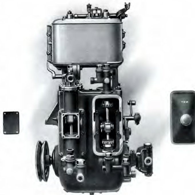
FIG. 9. LEFT SIDE OF THE WHITE STEAM ENGINE, WITH PUMP COVERS REMOVED
